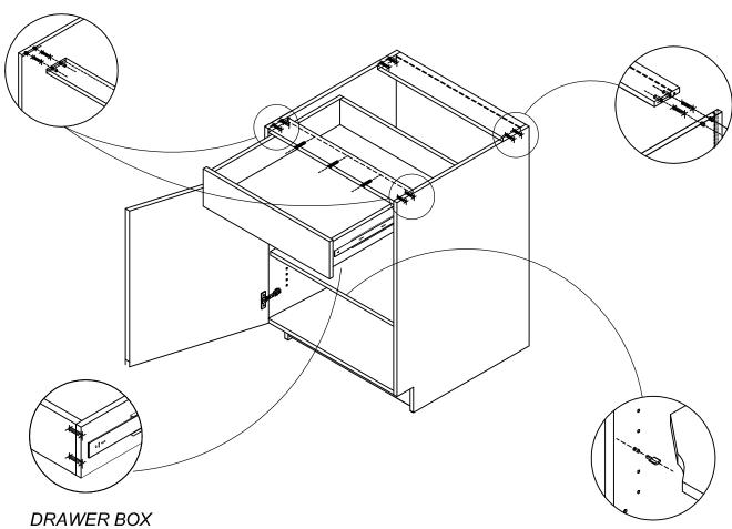
5/8" laminated box with Melamine finish Dowel joint construction Full extension ball bearing guides
